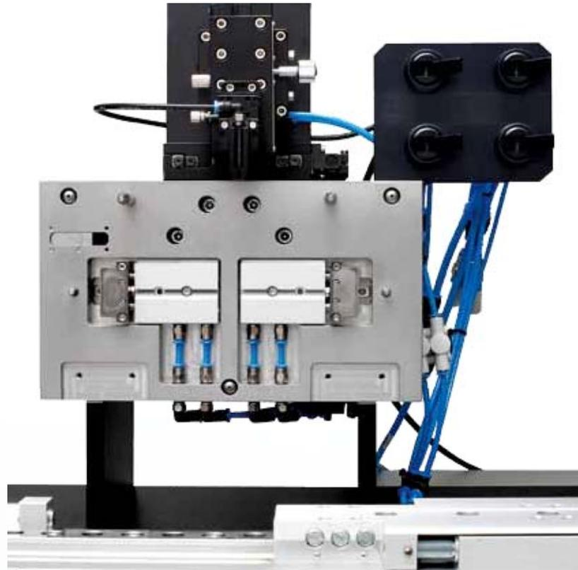
Loading stations outside of the system are used for mounting the work pieces. This reduces the process time to the core process and increases the throughput.
