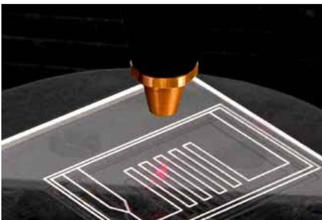
VersaWeld-TLPW focuses the beam strongly to obtain very fine weld seams.
