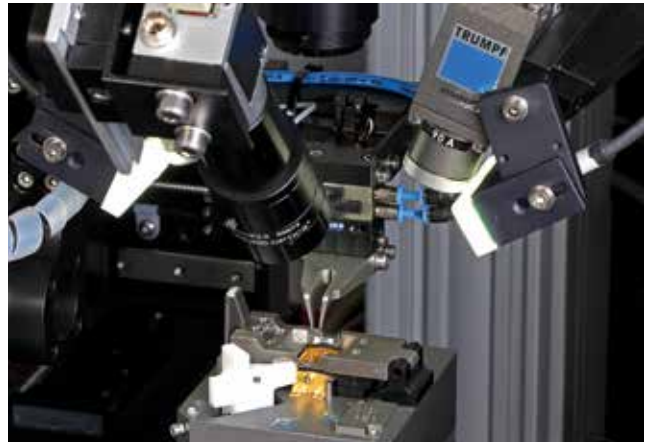
A CCD camera mounted on the focusing lens supports the image data processing during laser welding.
