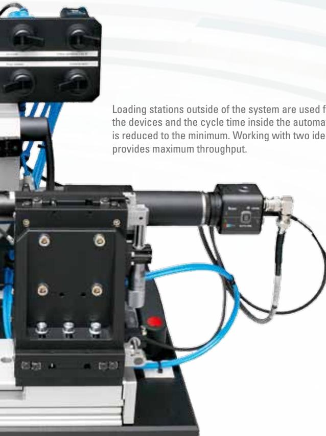
Loading stations outside of the system are used for mounting the devices and the cycle time inside the automated station is reduced to the minimum. Working with two identical trays provides maximum throughput.
