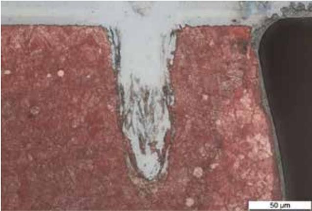
The cross section shows the welding penetration of a Kovar lid to a copper baser with a pulsed fiber laser when purging with protective gas.
