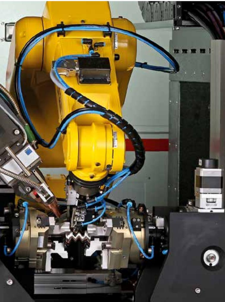
Customized configurations of the VersaWeld System replace tedious manual or semi-automated processes. Robots load the piece parts and can hold them in place during laser welding. With automated seam tracking, the position of the weld beam follows the calculated path for optimum welding results.
