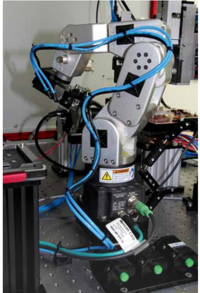
The NanoRobot precisely handles small parts in the VersaWeld station. Repetitive movements are executed with an error of less than 5  $\mu\text{m}$ . This performance qualifies the robot for direct placement of workpieces under the weld beam as well as for part inspection in machine vision stations for a visual assessment. NanoRobot has 5 N load capacity and a working range of 300 mm.
