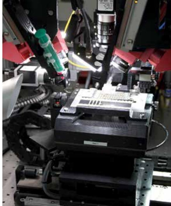
Selective laser soldering works with pre-tinned devices or solder paste. Two symmetric optical heads introduce a balanced energy and avoid unwanted shift.
