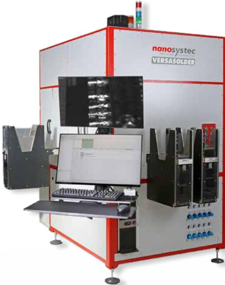
Feeders allow for unattended and fully automated operation except for cassette loading and unloading.
