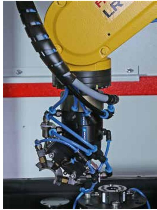
Loading with robots includes automatic tooling changes in order to provide maximum versatility. In this way, multiple process steps or different products will be processed without operator intervention.
