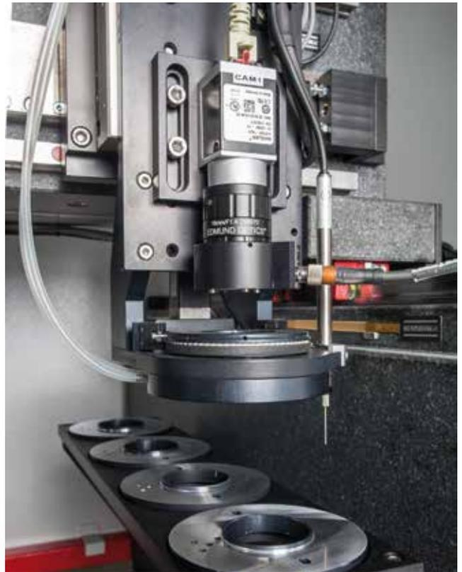
Different toolings can be changed during the process without operator intervention.
