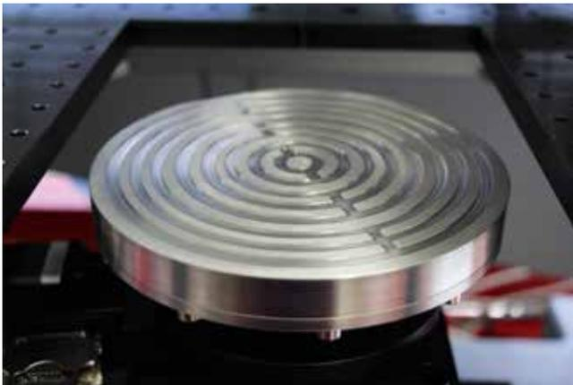
The wafer chuck presents various vacuum zones which can be activated as necessary. Combined with the excellent flatness over the chuck surface, the wafers are securely held without any distortion.
