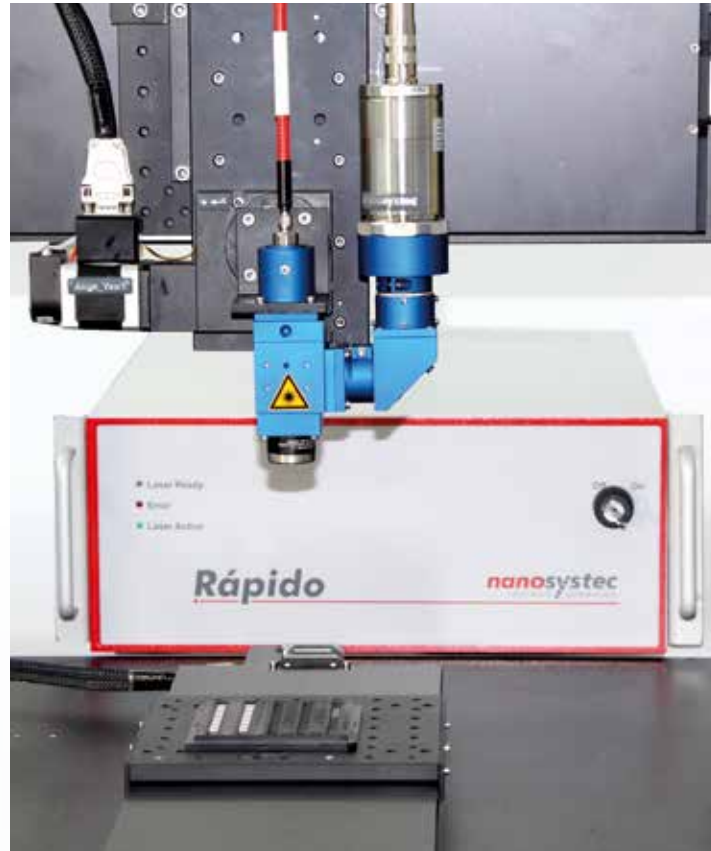
Rápido Blue provides an integrated pyrometer which measures the temperature in the solder joint with high accuracy and adjusts the optical power within milliseconds.
