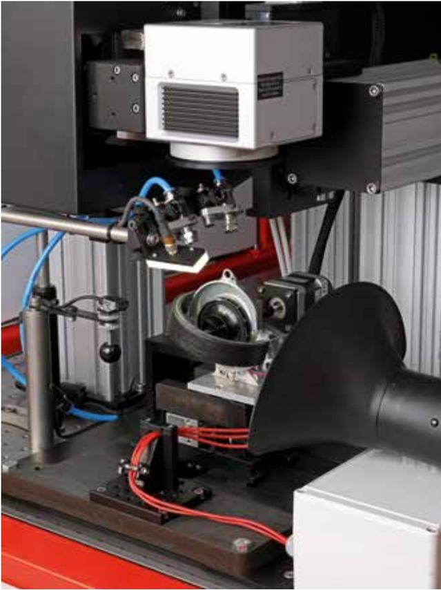
Fixtures with quick loading mechanisms support the efficiency of NanoBalancer.
