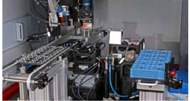
Multiple device trays and stop-motion conveyor belts increase the throughput and allow for the integration into fully automated production lines.
