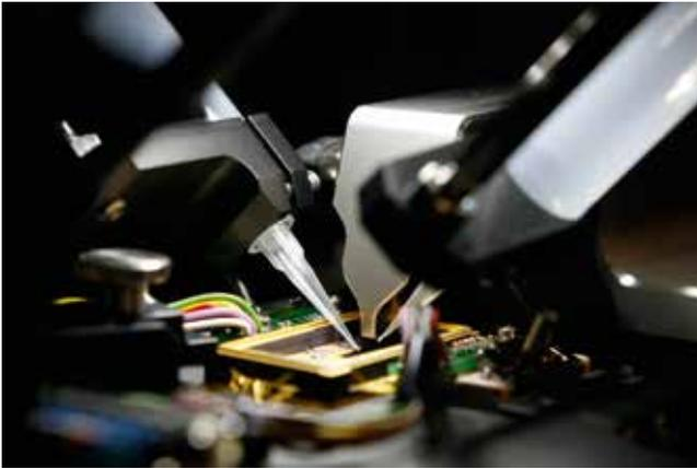
The entire process of alignment, resin dispensing and curing runs fully automated.
